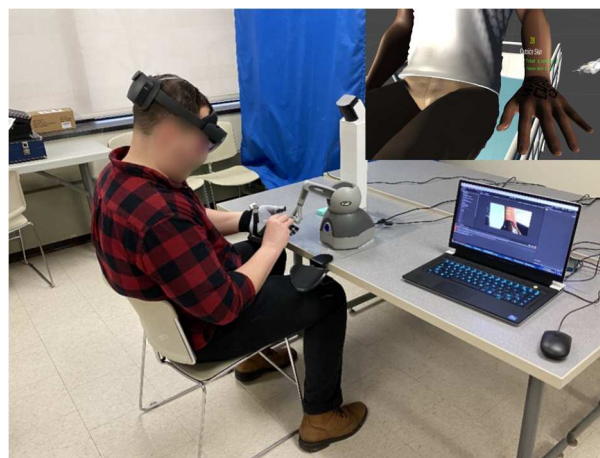
Fig. 3. A participant using the HMR IV Needle Insertion Simulation system during the experiment.
